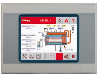
Through a MODbus connection, SPECTOR*control* is able to communicate with the automatic firing systems of leading manufacturers. All data are displayed on the monitor, and admissible parameters can be set. This represents one of the special strengths of the system: everything on just one user interface — the boiler attendant need not concern himself with different systems and is able to see both water data and burner data on a single device.
